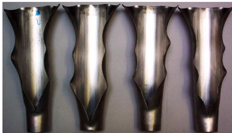
Fig. 3. Tubes split with unsymmetrical conical die.
